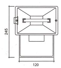
This fitting can be locaterd internally (as an up lighter) or externally (to provide flood lighting). This fitting is rated IP65.
