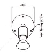
This version of the Gary employs a GU10 mains voltage lamp which eliminates the need for a transformer. It is surface mounted on a plate and is slightly larger than the 12v Gary (due to a larger lamp holder). It is finished in brushed aluminium,. Available in single, double and triple versions.
