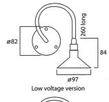
SKK Gooseneck lights are ideal for reading in bed without disturbing a partner who is sleeping. The lights are wall mounted and are fully adjustable using their gooseneck. The dimmable version shown also gives control of the light level through an integral push-button switch. The fitting is available as a mains voltage version, longer necks can be incorporated at additional cost.
