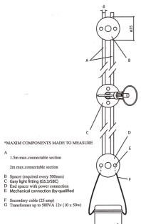
The track system uses solid brass flat sections to conduct low-voltage power to the lamps. The system is easy to use and is versatile in its application. It can run in a vertically curved sectional space and is supplied in natural brass or satin chrome.
