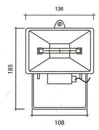
This discreet mimi-uplighter can be used internally and externally for accent lighting on walls and general flood lighting in confined areas. This fitting is rated IP65.
