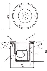
This is an LED version of the Walk On Me which has particurarly useful applications. LEDs are very energy efficient with a lanp life of 50,000 hours (approx). The lamp also remains much cooler than halogen during use (surface temperature approx. 5C). This fitting is available in blue, white, red, green and yellow. It is used as a feature light rather than large-scale wall washer. This fitting has a rating of IP65. It must be earthed and wired to a circuit breaker. NOT DIMMABLE
