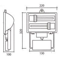
The PL up lighters are designed for office lighting where running costs and maintenance are a priority, the fittings can be adapted to be used externally, the ballasts are located in a remote aluminium enclosure below the fitting or in a remote location. This fitting is rated IP65.
