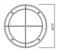
The bulhead is an external weather-proof wall-mounted fitting available in three models: plain, cross and eyelid. The plain version gives maximum illumination whilst the cross and eyelid are more protected and offer an alternative esthetic. An emergency version is available. This fitting is rated IP65.
