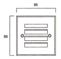
The SKK Nightlight is perfect for lighting stairs and walkways at skirting level. The fitting has a louvered face plate to direct the light down and minimise glare. The low-voltage capsule lamp version can be used for both dramatic and subtle effects.
