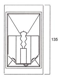
This compact wall-mounted uplighter is very discreet and economises on space whilst casting a good level of light on to the ceiling. The fitting can be used alone or in conjunction with the classic SKK corner uplighter. The fitting is cast aluminium and can be painted to match the wall colour and is available with a glass cover.
