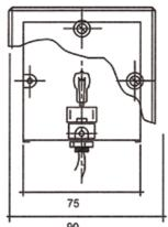
This lamp provides a soft, diffused light at floor level. There are two models in this range; the square skirting with an etched-glass square block and the square skirting stainless steel (SS) which incorporates a sealed etched-glass rectangle that resists moisture.
