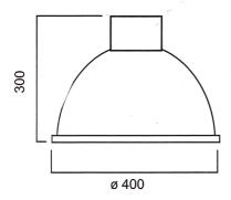
The High Bay is a suspended "loft-style" aluminium lamp shade. Additional components available include a ceramic lamp holder and Pendant set.
