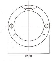
The par 36 is a fixed low-voltage downlighter. The sealed lamp allows it to be installed in areas where cleanliness and water resistance is important such as catering applications, bathrooms and semi-external locations. WFL lamp pictured.
