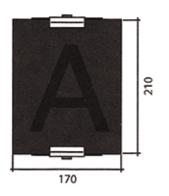
A simple light that can be surface mounted or semi-recessed. The glass panel can be engraved, coloured or etched to a design of your specification, for an additional charge.
