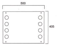
This surface-mounted bathroom mirror has four frosted circular light points along either side, which can be customised in shape and size at additional cost.
