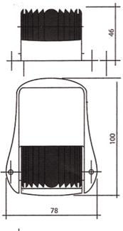
a remote transformer. The stern is weather resistant so therefore is excellent for long-lasting application in wet areas whether internal or external. Thois fitting is directional and is rated IP65.
