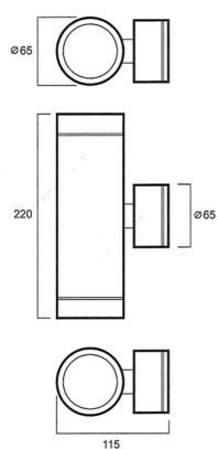
This exterior wall light provides direct illumination in two directions (up & down), and is perfect for highlighting either side of external dorrways. The fitting is extremely durable, and can be installed quickly and easily without the need of a transformer. The fitting is available in antique bronze, aluminium and brass finishes.
