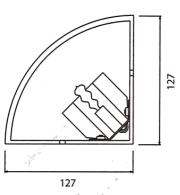
A surface mounted uplighter that can be mounted into the corners of a room. It is discreet and economical on space (enabling walls to display pictures rather than conventional uplighters) but still casts good light on to the ceiling. The finish is raw aluminium and can also be finished in the colour of the room.
