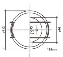
Surface mounted integral halogen light using a 50w PAR396 lamp is a glare proof bulb with the filament totally sealed. Ideal for kitchen, bathroom and general lighting applications.
