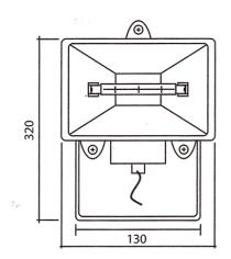
This exterior fitting can be used in locations where genreal flood lighting is required. The UP300XL has the highest output of all the exterior up lighters and has the widest coverage from the spectacular reflector. It can also be used inside as an uplighter. This fitting is rated IP65.
