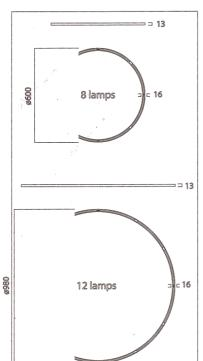
The Halo Ring is a light-weight minimal chandelier solution available in two standard sizes; a 600mm diameter version incorporating eight 5w lamps and a 980mm version incorporating twelve 5w lamps. The Halo Ring can also be made to custom configurations.
