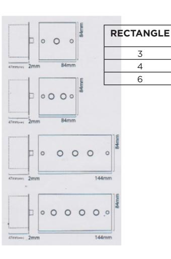
Intermediary switches are available for super switches on request, at additional cost.
