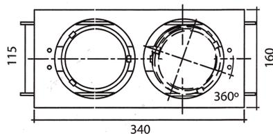
The trayspot incorporates two 20/50w halogen lamps, taking current from the barewire system. Ideally suited for exhibition and display environments where soft lighting is essential. Can be used individually or grouped for required effect.
