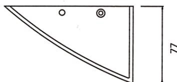
A surface mounted uplighter that can be mounted into the corners of a room. It is discreet and economical on space (enabling walls to display pictures rather than conventional uplighters) but still casts good light on to the ceiling. The finish is raw aluminium and can also be finished in the colour of the room.
