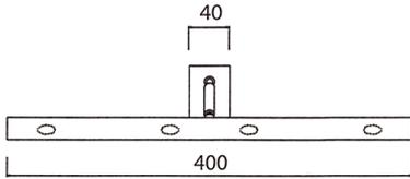
A simple, streamlined tubular fitting sold in 4 lengths ; 300mm, 400mm, 600mm, 800mm. Finishes come in brass, antique bronze (light or dark), chrome or nickel. For use with a remote transformer (100w max) in a double bisa box. NB Customised length up to 1 metre.
