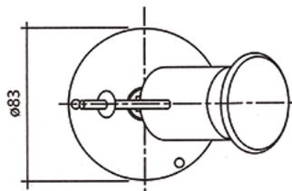
This fitting is adjustable to 360 degrees in the horizontal plane and 90 degrees in the vertical. As the lamp operates at mains voltage it can be used in locations where transformers cannot be accommodated. The fitting is available for use with GU10 lamps, and is also available as a twin version (202).
