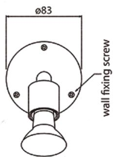
This version of the Gary employs a GU10 mains voltage lamp which eliminates the need for a transformer. It is surface mounted on a plate and is slightly larger than the 12v Gary (due to a larger lamp holder). It is finished in brushed aluminium. Available in single, double and triple versions.
