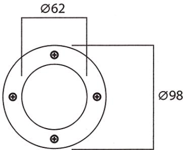
This larger mains voltage version of the HP500 is ideal for areas where transformers cannot be accommodated. The fitting is waterproof. Available in natural aluminium, stainless steel and antique bronze finishes.
