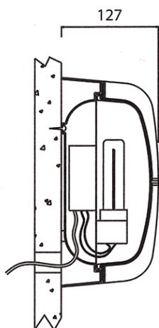
The bulhead is an external weather-proof wall-mounted fitting available in three models : plain, cross and eyelid. The plain version gives maximum illumination whilst the cross and eyelid are more protected and offer an alternative esthetic. An emergency version is available. This fitting is rated IP65.
