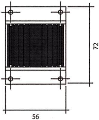
The stern is a low-voltage fitting giving diffused light using a remote transformer. The stern is weatherproof so therefore is excellent for long-lasting application in wet areas whether internal or external. This fitting is rated IP65.
