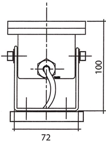
The HP500 waterproof external fitting is ideal for garden or landscape lighting. The small size allows the fitting to be discreetly located, including bushes or around tree bases. The fitting is rated IP65 and is available in natural aluminium, with accessories including an external transformer (rated IP65) and HP500 spike. (see picture). The HP500 is also available as an LED version - see 'LED' section. See page 5 for LED version.
