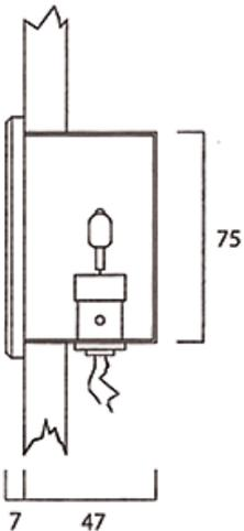
The SKK Nightlight is perfect for lighting stairs and walkways at skirting level. The fitting has a louvered face plate to direct the light down and minimise glare. The low-voltage capsule lamp version can be used for both dramatic and subtle effects.
