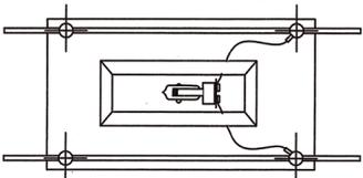
This fitting was originally developed for the V&A's Twentieth Century gallery in London. Designed for an insulated wire system, the luminaire provides reflected illumination from the ceiling. This is ideal for office lighting and environments where reflection from light sources on computer screens is of concern.
