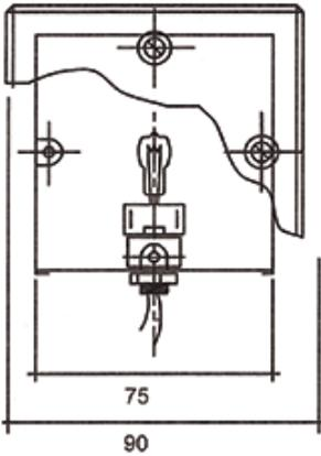
This lamp provides a soft, diffused light at floor level. There are two models in this range ; the square skirting with an etched-glass square block and the square skirting stainless steel (SS) which incorporates a sealed etched-glass rectangle that resists moisture.
