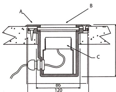
This is an LED version of the Walk On Me which has particularly useful applications. LEDs are very energy efficient with a lamp life of 50,000 hours (approx). The lamp also remains much cooler than halogen during use (surface temperature approx. 5C). This fitting is available in blue, white, red, green and yellow. It is used as a feature light rather than large-scale wall washer. This fitting has a rating of IP65. It must be earthed and wired to a circuit breaker. NOT DIMMABLE
