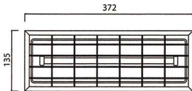
This is an emergency light fitting housed in a galvanised steel protective box. The lamp is a T5 fluorescent and the fitting includes an integral 3 hour battery pack.
