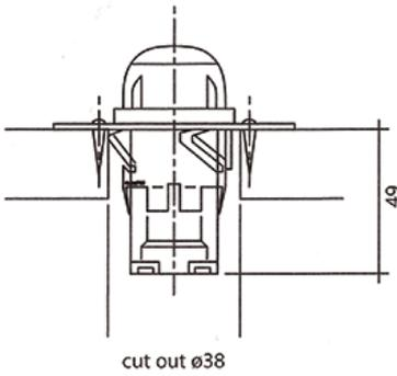
The oven round light is available in three styles: round, flat and large flat (round glass shown in main image). The fitting is recessed in the wall and can be fitted into a deeper bise box. It can be used either as a ceiling or wall luminaire (particularly at skirting-board level).
