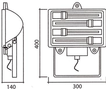
The PL up lighters are designed for office lighting where running costs and maintenance are a priority. The fittings can be adapted to be used externally. The ballasts are located in a remote aluminium enclosure below the fitting or in a remote location. This fitting is rated IP65.
